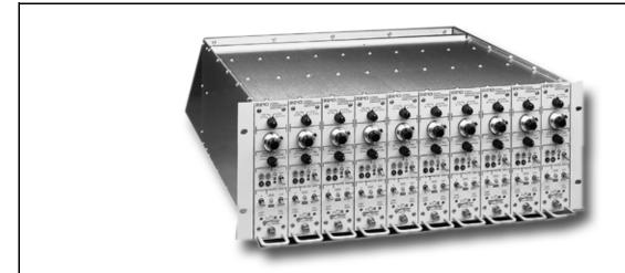
Model 2250A rack adapter allows assembly of signal conditioning amplifier modules for multi-channel testing. Ten-channel system shown in rack. All wiring is built-in to accept adjacent ten-channel systems.
